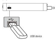
(Sample Illustration) Connecting a USB device
